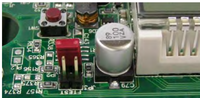
• Figure 7-13 Location of the Config jumper
